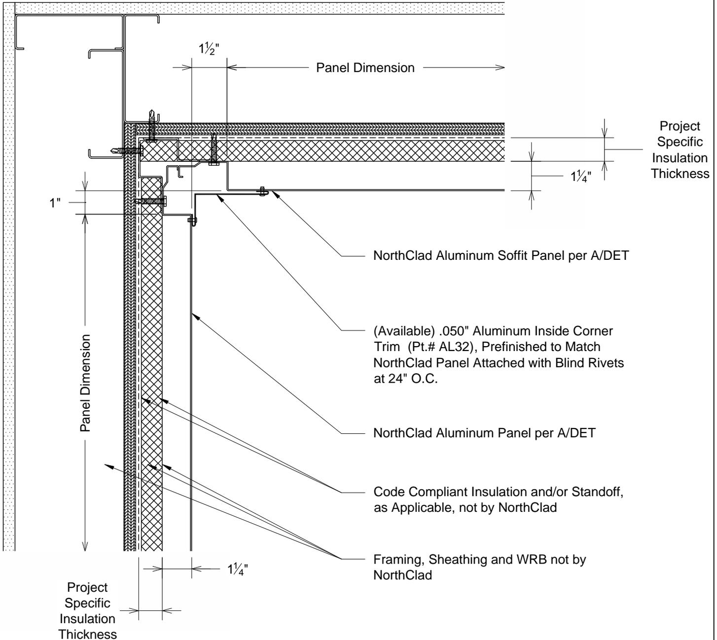
Q1 Section - Soffit at Top of Wall
