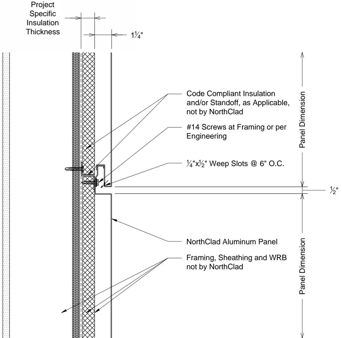
A Section - Horizontal Joint
