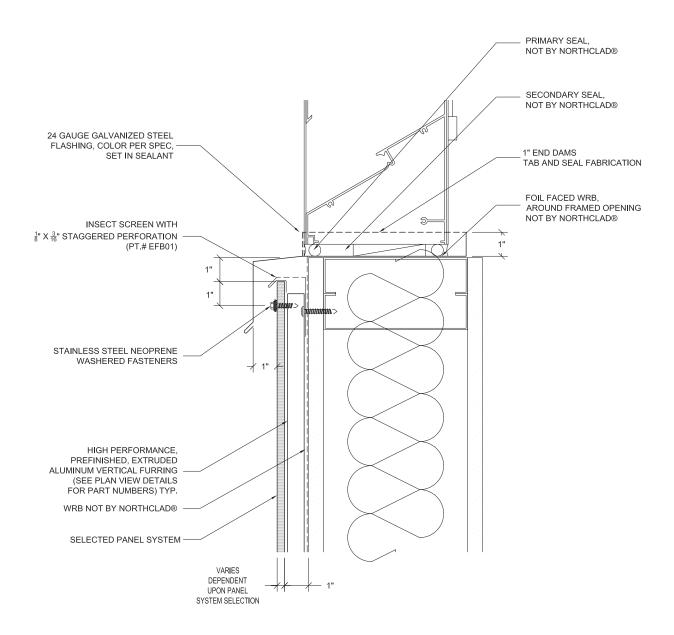
For details without exterior insulation, or to download the CAD version of this detail, please see www.northclad.com.
