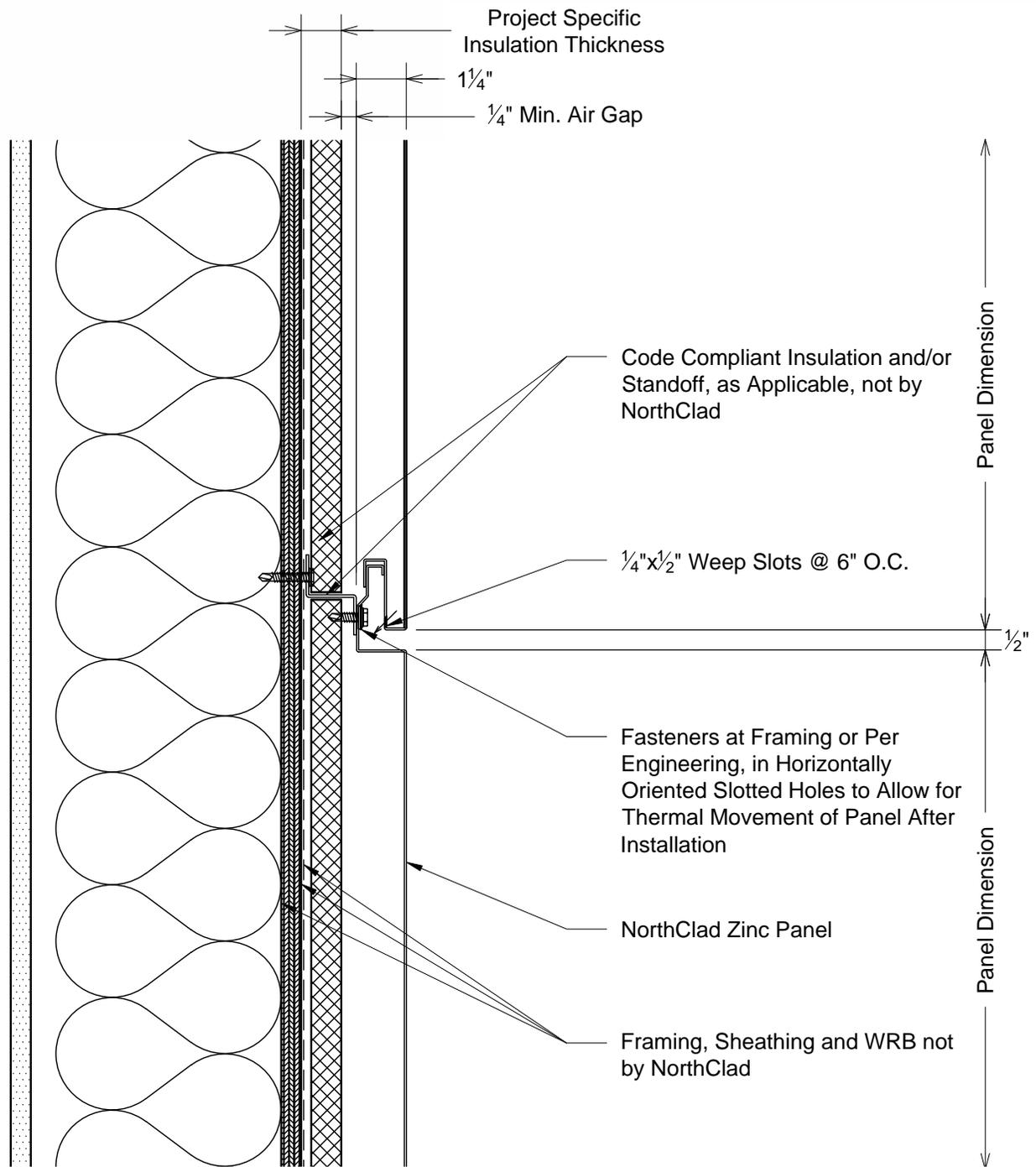
A Section - Horizontal Joint
