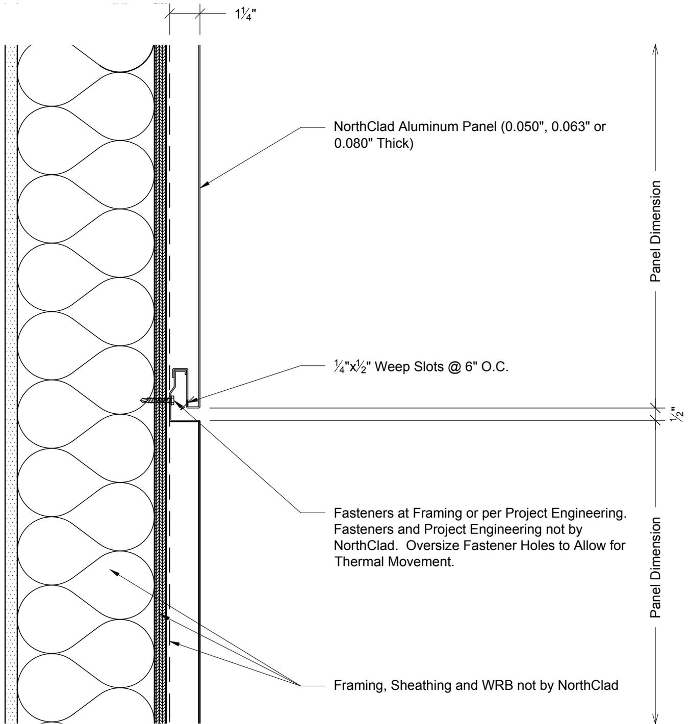
**A** Section - Edge of Panels at Horizontal Joint
