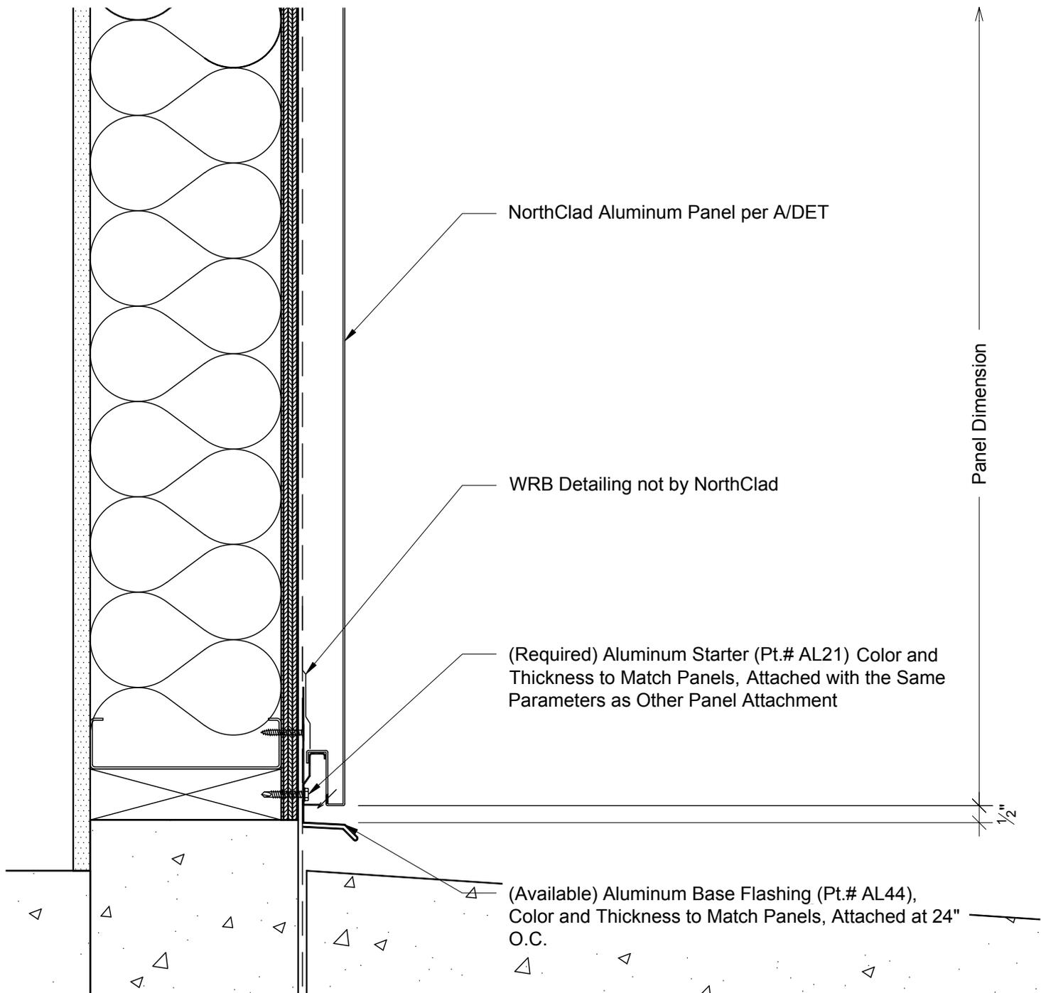
**C** Section - Bottom of Panel at Base of Wall
