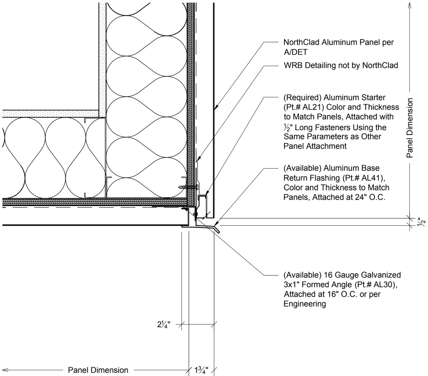
**M2** Section - Panels at Soffit to Fascia Transition
