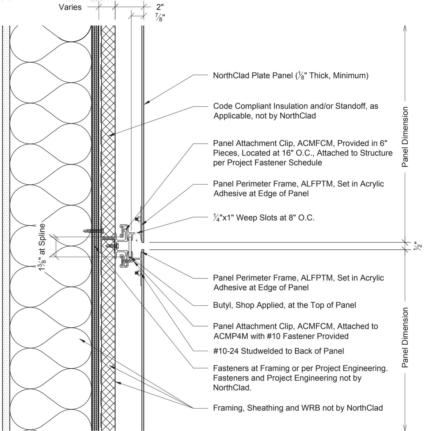
**A1** Section - Edge of Panels at Horizontal Joint
