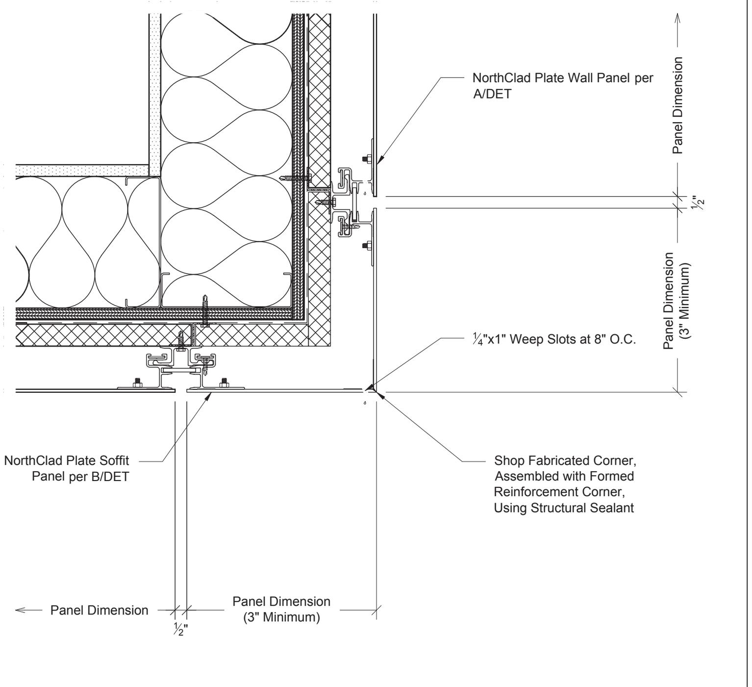
**M1** Section - Panels at Fascia to Soffit Transition
