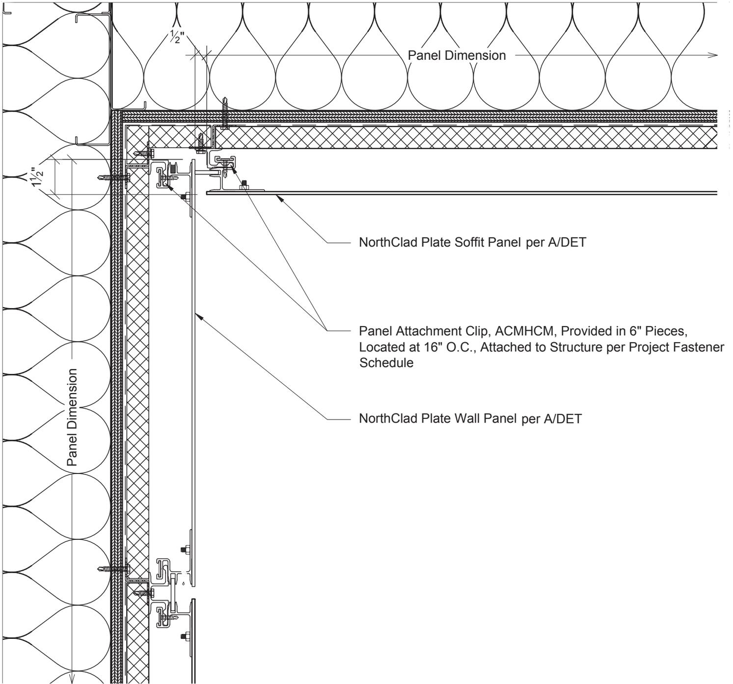
**N1** Section - Panels at Wall to Soffit Transition
