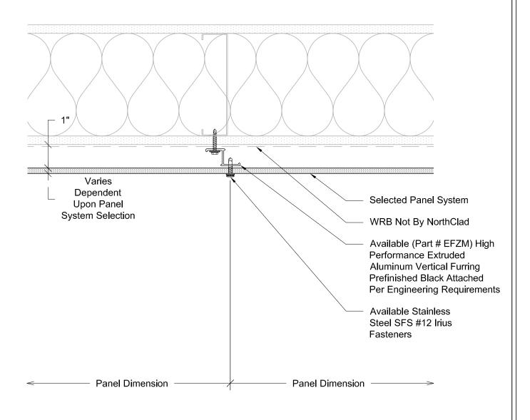
C Plan View - NorthClad EF - Vertical Fastener
