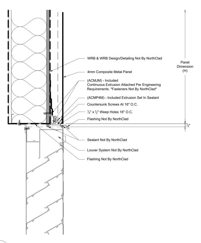
Section - NorthClad ACM - Framed Opening Louver Header
