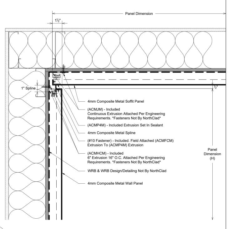
Section - NorthClad ACM - Soffit to Wall Inside Corner
