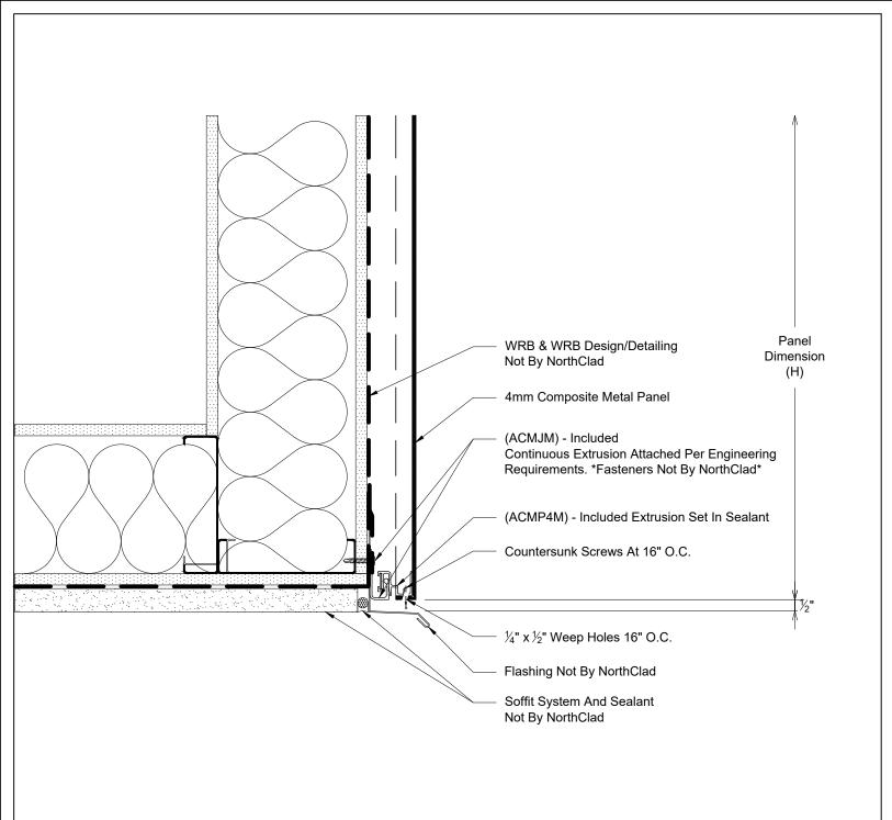
Section - NorthClad ACM - Fascia to Soffit by Others
