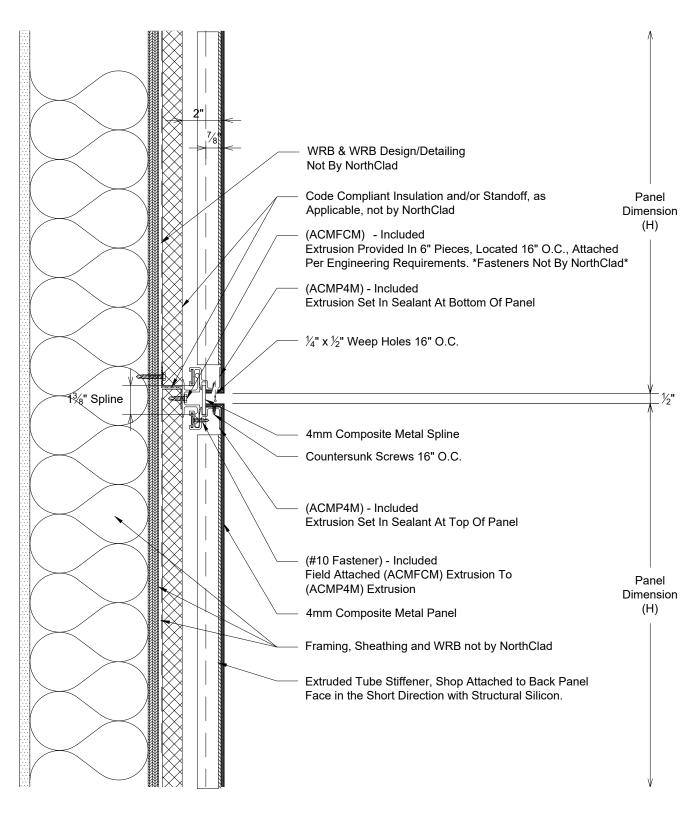
Section - Horizontal Joint System: NorthClad ACM System on Outboard Insulation
