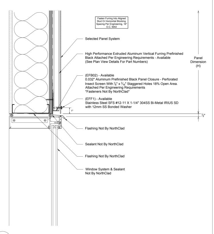
Section - NorthClad EF - Framed Opening Window Header
