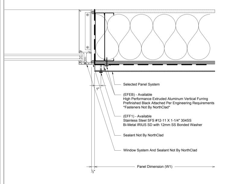
Plan - NorthClad EF - Framed Opening Window Jamb
