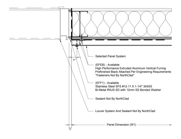
Plan - NorthClad EF - Framed Opening Louver Jamb
