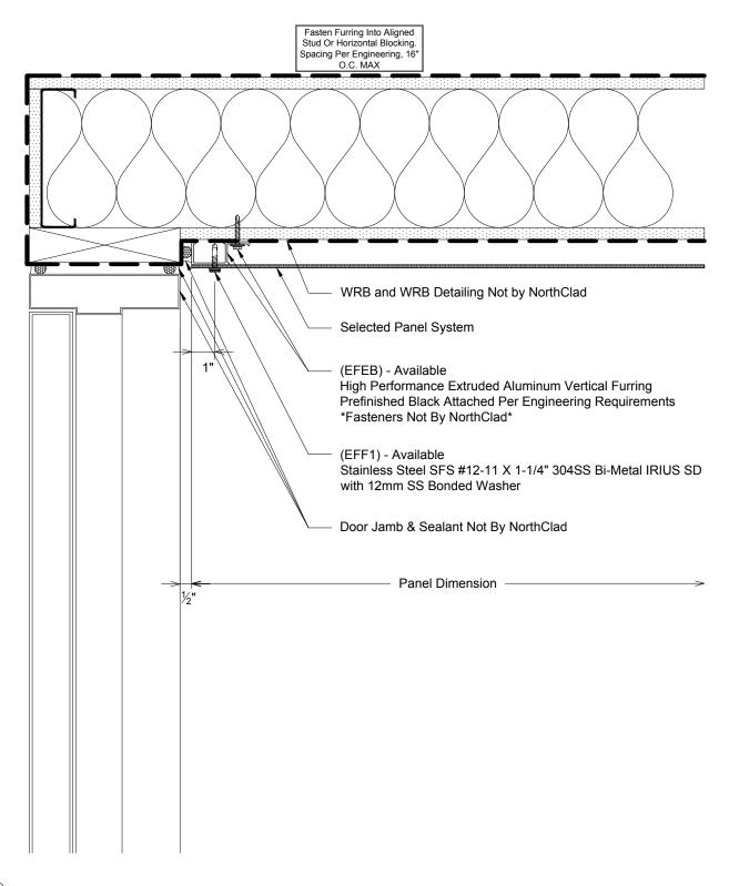
Plan - NorthClad EF - Inside Corner to Jamb
