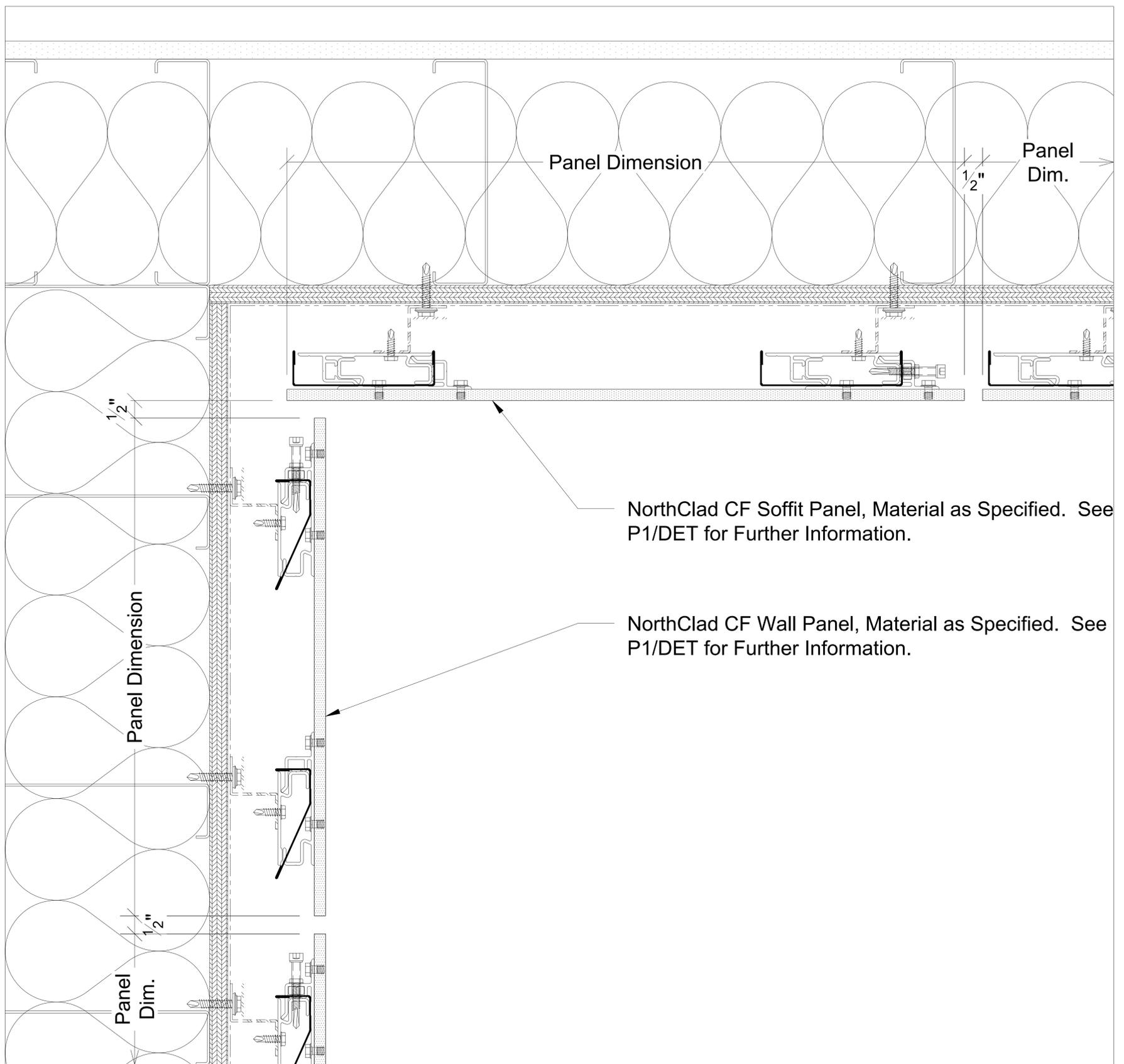
NorthClad CF Soffit Panel, Material as Specified. See P1/DET for Further Information.
