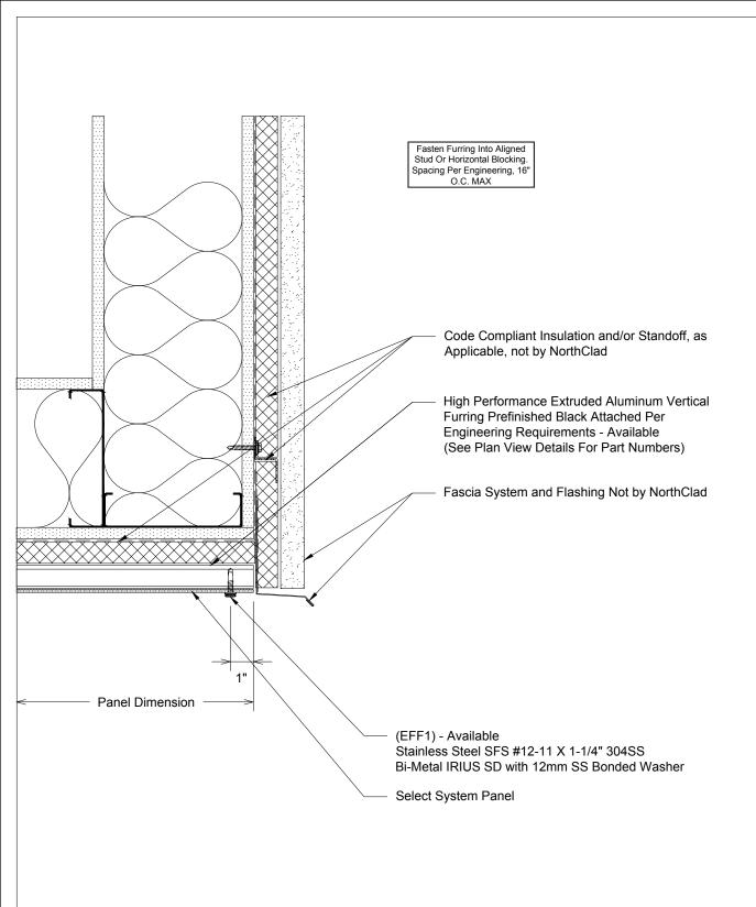
Section - NorthClad EF - Soffit to Fascia by Others
