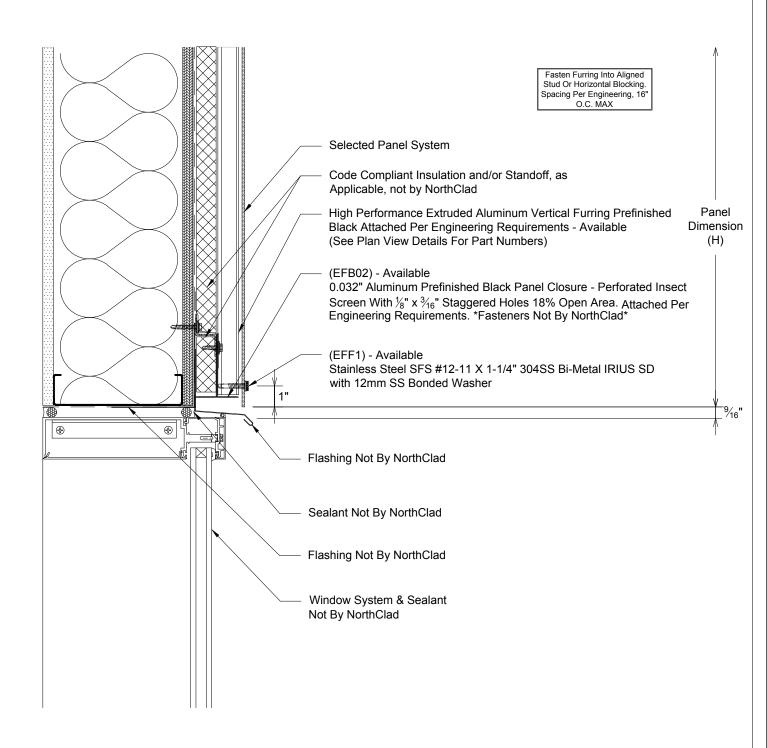
Section - NorthClad EF - Framed Opening Window Header
