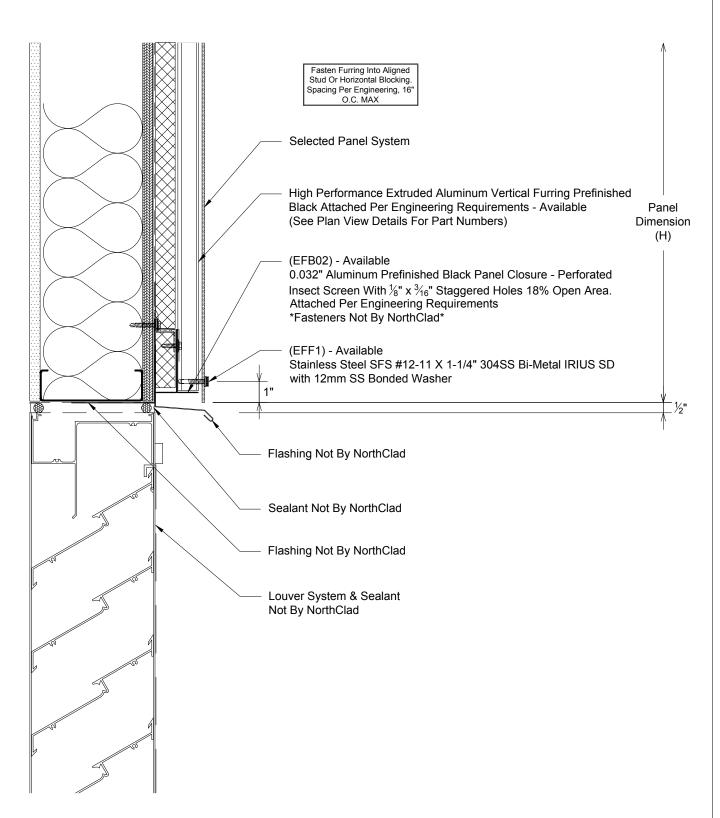
Section - NorthClad EF - Framed Opening Louver Header
