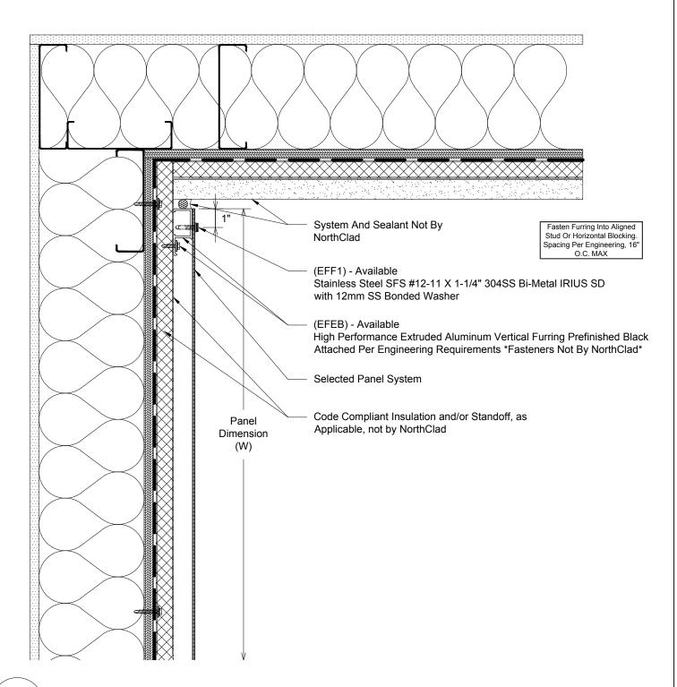
Plan - NorthClad EF - Inside Corner Termination
