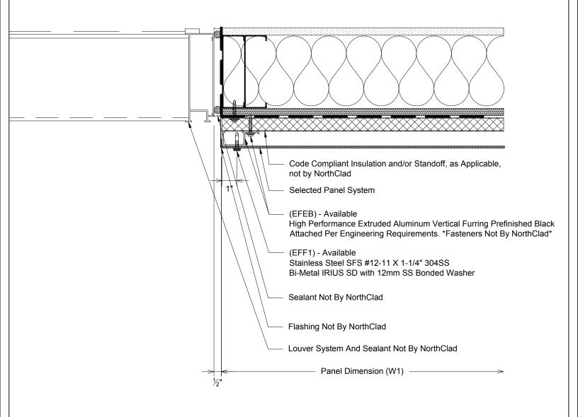
Plan - NorthClad EF - Framed Opening Louver Jamb
