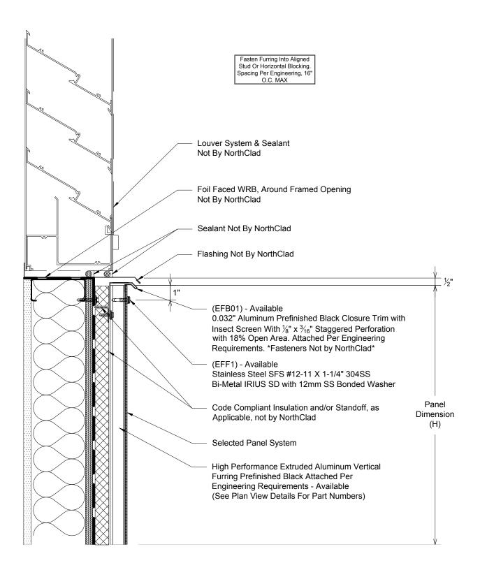
Section - NorthClad EF - Framed Opening Louver Sill
