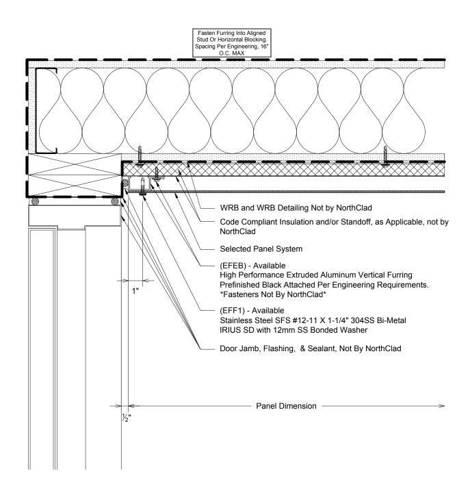
Plan - NorthClad EF - Inside Corner to Jamb
